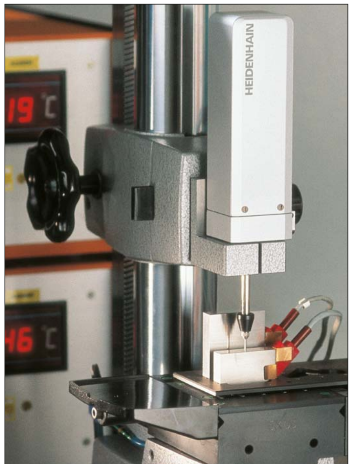
Calibration of gauge blocks
