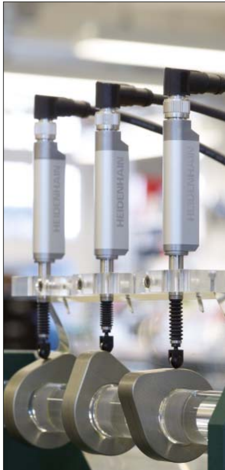
Testing station for flatness inspection
